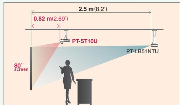
The PT-ST10U, which is equipped with the newly developed short-throw lens, lets you project images onto a large, 80-inch screen from a distance of only 0.82 m (2.69'). This greatly increases the projector's range of use.
