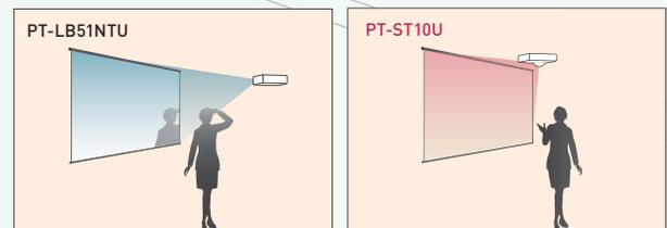
The close range projection of the PT-ST10U reduces the chance of the presenter standing in front of the projection light and casting a shadow on the screen. Also, presentations are more comfortable because the presenter is not affected by the glare of the projection light.
